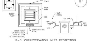
IP-5. OVEREXCAVATION INLET PROTECTION
