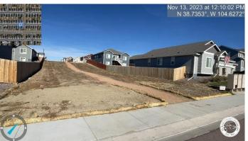
Photo 15: Failure to stabilize and achieve uniform vegetative cover with an individual plant density of at least 70 percent.
